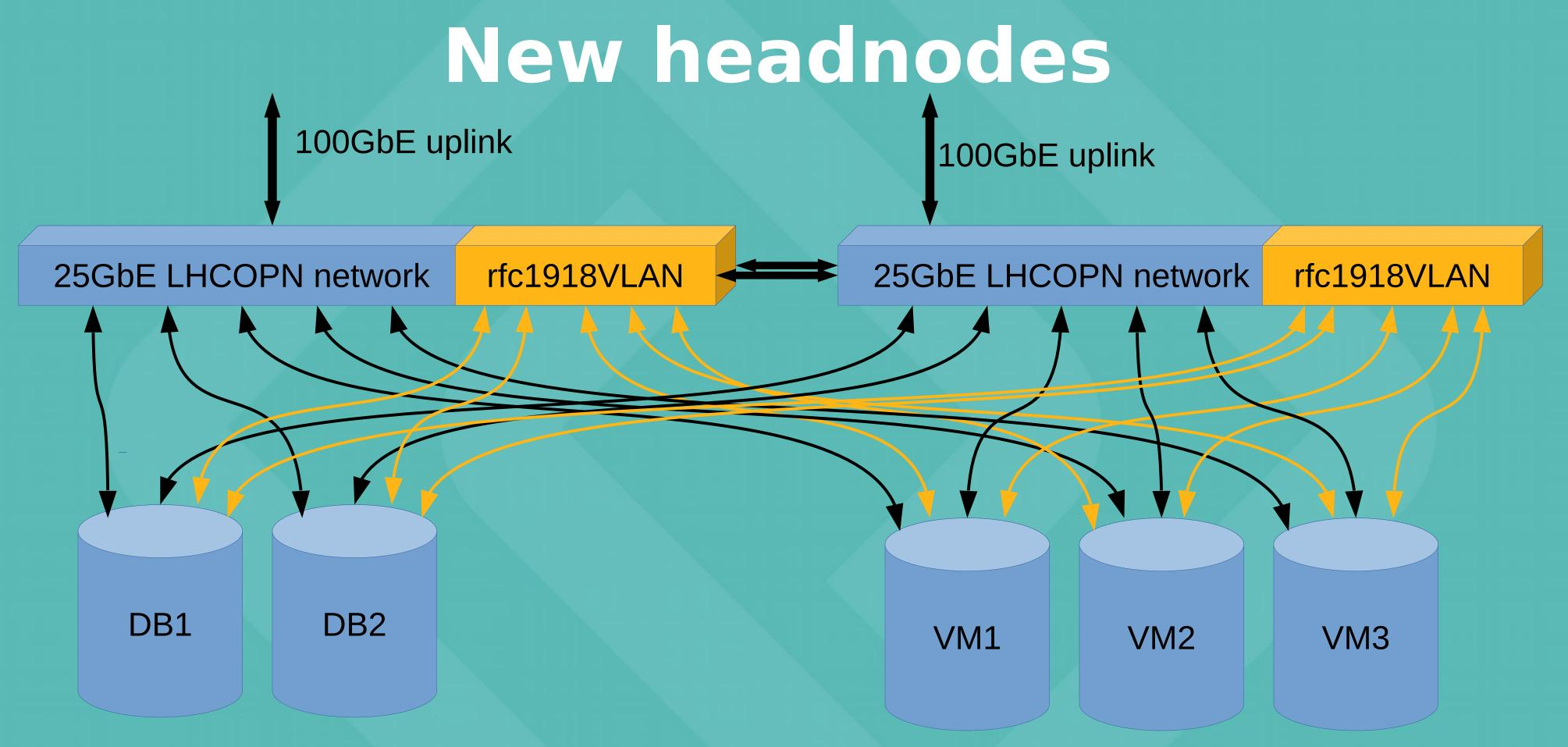
5 x Dell r640 with 2x5222 (2x4 core 3.8GHz) and 192GB RAM, 2TB SSD 4x25GbE for redundant (LACP) internal and external network Network 2xS5212F-ON (12x25+3x100) with multi-chassi link aggregation
